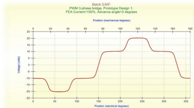
Fig.13. BACK EMF vs. POSITION (electrical degree)
