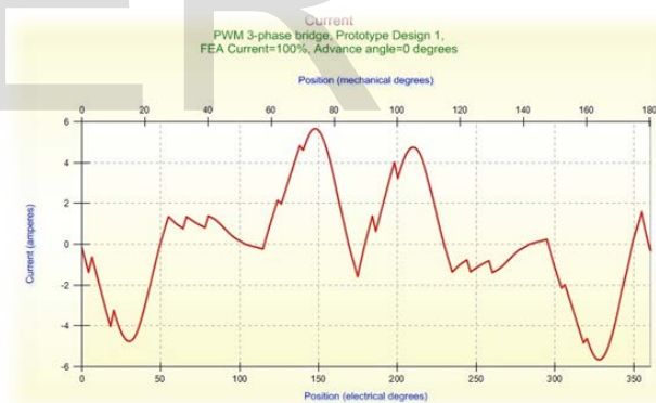
Fig.12. Current vs position(electrical degree)
